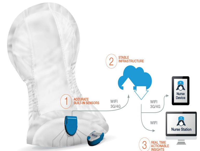
Figure 1: Abena Nova, the intelligent incontinence product for everyday use 1. ACCURATE BUILT-IN SENSORS: Residents wear an Abena Nova continence product with imprinted sensors and a small attachable clip. 2. STABLE INFRASTRUCTURE: Data is transmitted to the cloud irrespective of the facility's physical environment and IT set-up. 3. REAL TIME ACTIONABLE INSIGHTS: Caregivers are notified (tablet, PC, smart phones) and take action.
